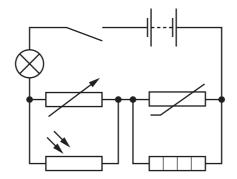
What is connected in parallel with the thermistor?
